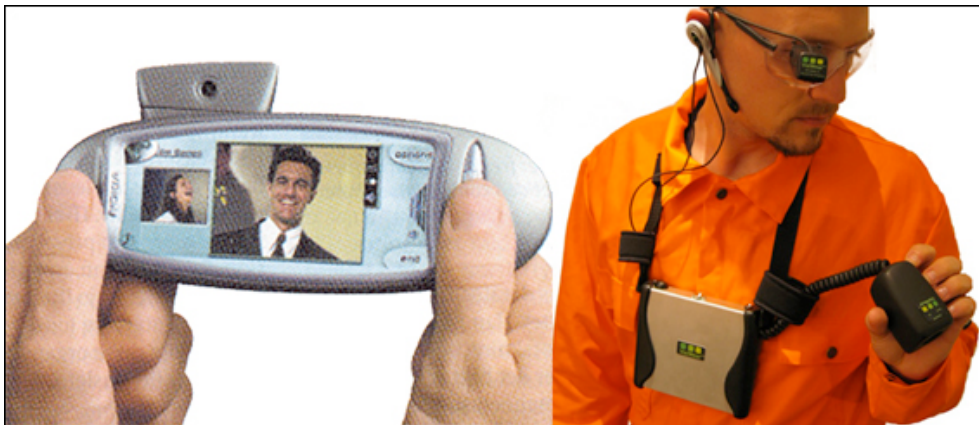
Figure 1 Left: Nokia’s implementation as a mobile (video)phone. Right: VisiWear’s implementation as a wearable computer
