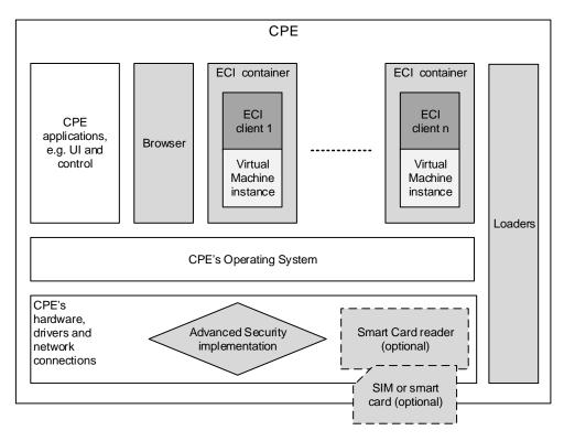
The figure shows the block diagram of a CPE with  $n \ge 2$  embedded ECI clients, each with their own Virtual Machine instance. The shaded areas are subject of this document and the planned specifications (B), (C) and (D). Optional elements are indicated by dotted lines.
