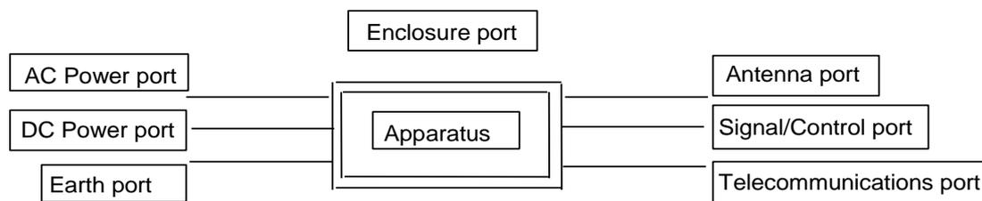
Figure 3.1-1: Examples of ports
