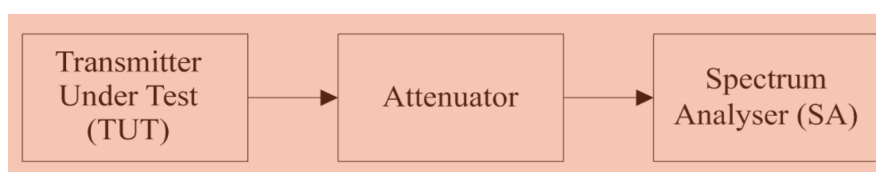
Figure 3: First adjacent channel power measurement (also applicable for symbol constellation error measurements)
