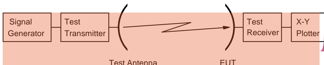
Figure 9: Test arrangement - antenna transmit radiation pattern measurement
