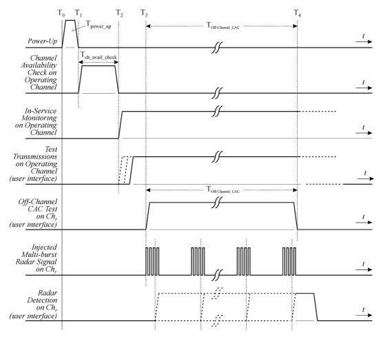
Figure 10: Example of timing for radar testing during the Off-Channel CAC
