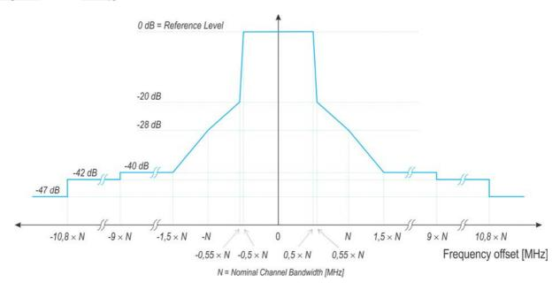
NOTE: dBc is the spectral density relative to the maximum spectral power density of the transmitted signal.
