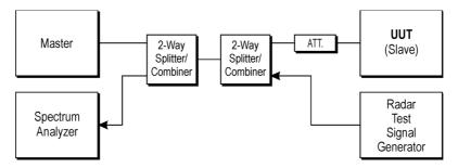
Figure 5: Set-up B
