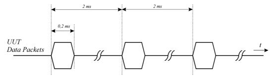
Figure 3: General structure of the test transmission sequences
