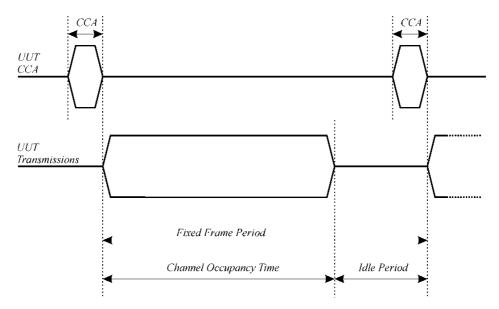
Figure 2: Example of timing for Frame Based Equipment
