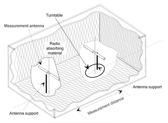
Figure B.3: A typical Fully Anechoic Room
