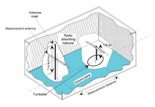
Figure B.2: A typical Semi Anechoic Room
