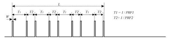
Figure D.3: General structure of a single burst/single pulse based staggered PRF radar test signal
