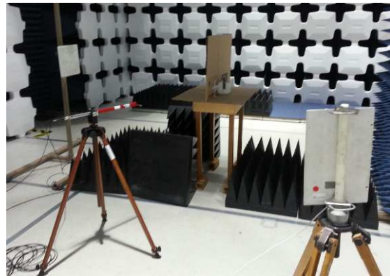
Fig 3 Configuration for measurement of interference GSM and RFID
