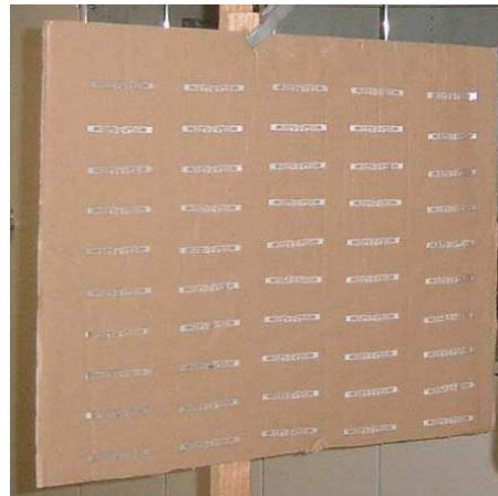
Fig 4 Photo of 50 tags mounted on cardboard sheet
