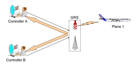
Figure 8: 2 controllers using a single frequency - example 1
