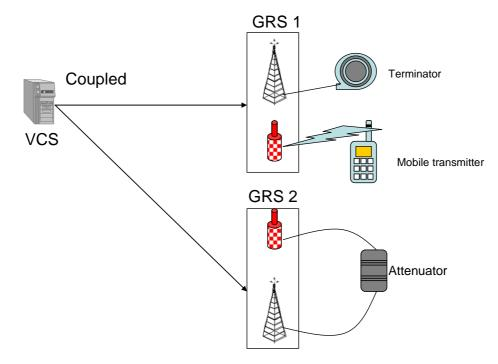
**Figure 5: test coupling infrastructure**
