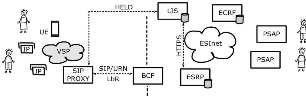
**Figure 6: Location by Reference (LbR) Test Configuration**
