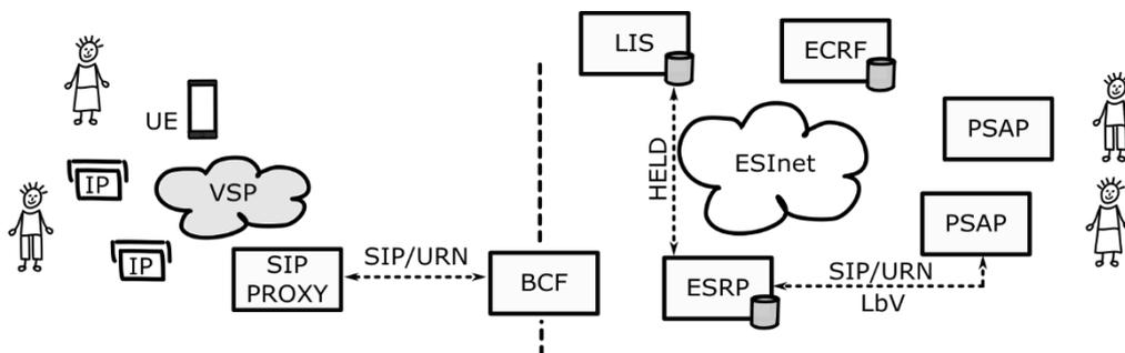
**Figure 7: Location by Value (LbV) Test Configuration**
