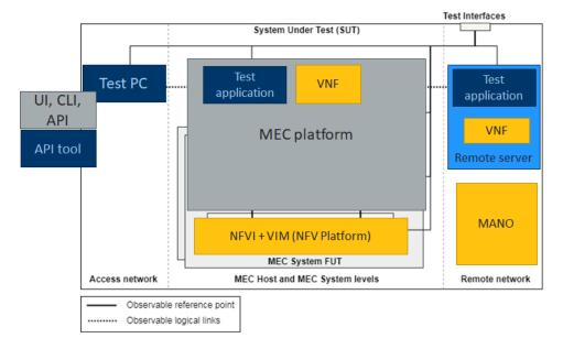
Figure 4. MEC Interoperability Testing
