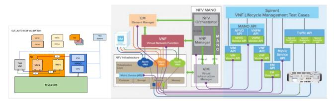
Figure 47. Demo 4: Test System for automated Life Cycle validation
