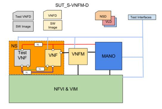
Figure 17. Specific VNFM (Direct Mode) Configuration: S-VNFM-D
