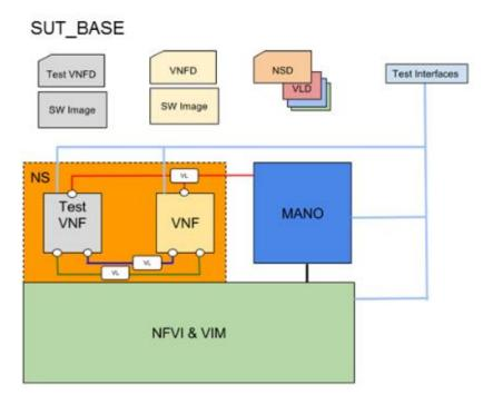
Figure 11. SUT Configuration example.
